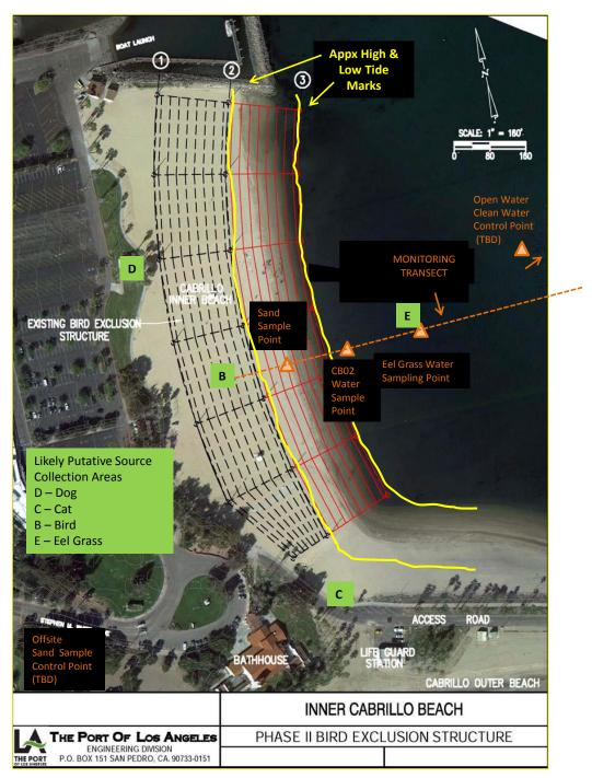
Figure 9. Conceptual Sanitary Survey Design Overlaying Proposed 2012 Expansion of Bird Exclusion Structure for Context
